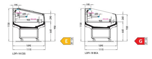
CSS – cover | single, straight | sliding (sideways) BCA – low glass or front glass riser | single, bent | fixed
